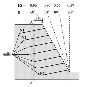
Figure 4. Excavation scheme and safety factors for different slope angles
