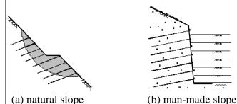
(a) natural slope (b) 1 Figure 1. Soil nailing applications
