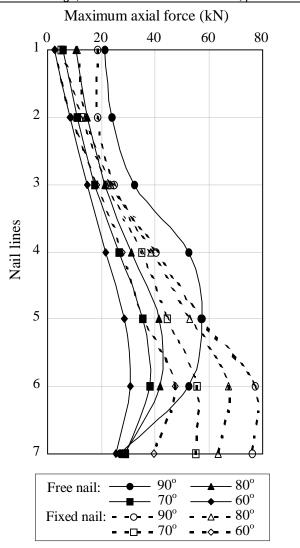
Figure 6. Maximum axial force on nail lines.
