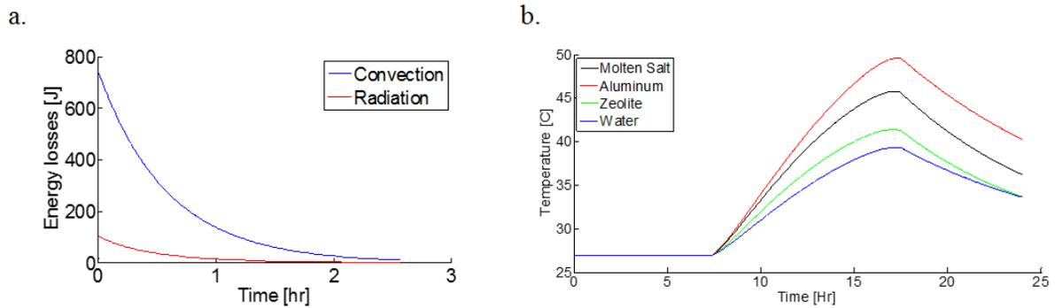
Figure 4. (a) Thermal storage energy decay due to convection and radiation. With no input of energy, a  $0.1\text{m}^3$  block of aluminum of  $0.1\text{m}^3$  takes 2.56 hours to go from  $100\text{ }^\circ\text{C}$  to  $25\text{ }^\circ\text{C}$ . (b) Maximum temperature for the same size thermal storage with standard solar irradiance, for different materials.
