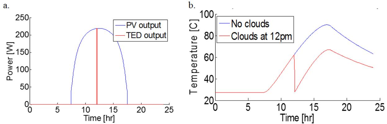
Figure 6. Behavior of a PV-TE system (M1), during an intermittency lasting 8 minutes that occurs at noon on 01/01/2014. (a) Shows the output power contributions by the PV and the TED. (b) Shows the temperature evolution of the Thermal storage, which decays during the intermittency by the TED using its stored energy.
