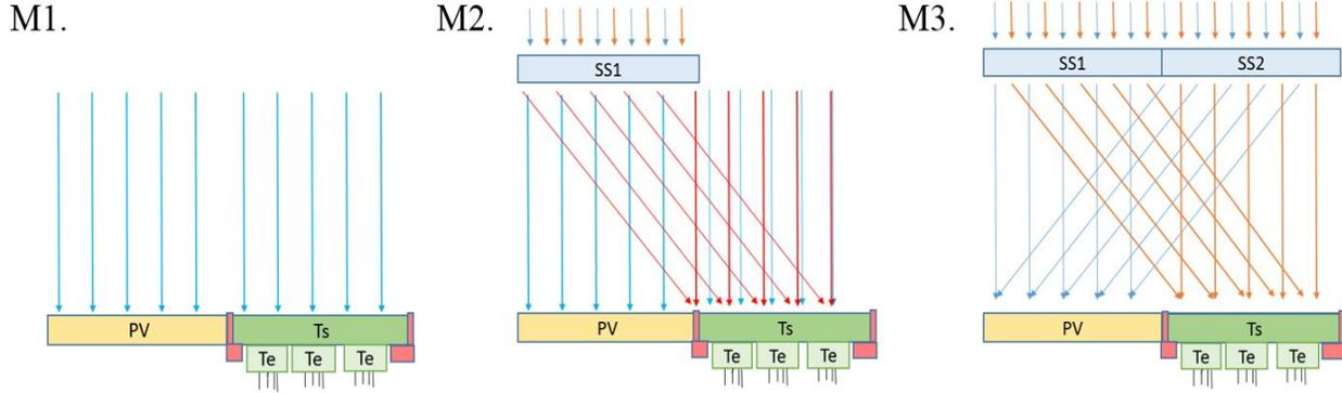
Figure 3. Three configurations for using the available solar illumination: Model 1 (M1) receives direct irradiance without spectral management, Model 2 (M2) uses partial spectrum splitting, and Model 3 (M3) uses full spectrum splitting.
