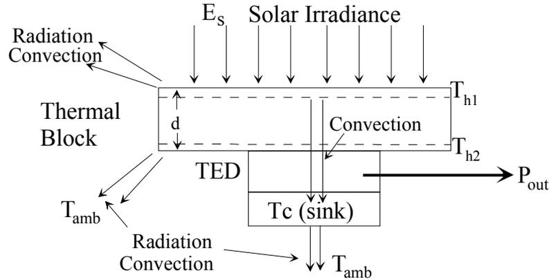
Figure 2. Detail of the input and output powers in a thermal block, with parameters affecting the heat transfer.
