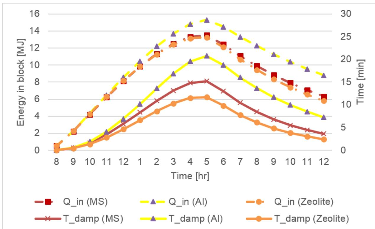
Figure 5. Energy available in the thermal storage at different hours throughout the day (M1). Different materials in a block of 1m<sup>2</sup> of surface area and 0.1m of thickness where simulated. The secondary axis shows the time an intermittency could be offset by the available energy.
