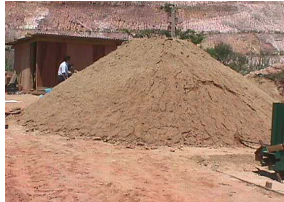
Figure 4: Soil Surcharge in a Pull-out Test
