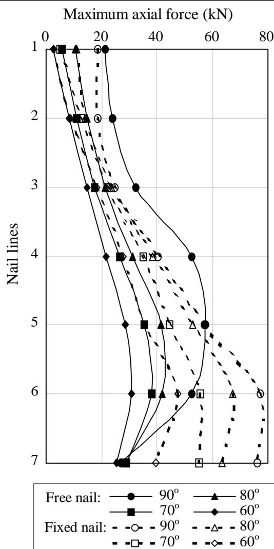
Figure 6. Maximum axial force on nail lines.
