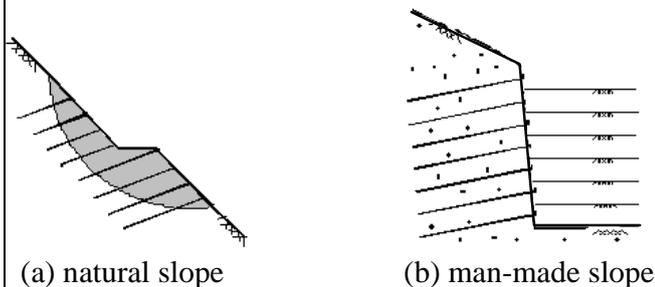
Figure 1. Soil nailing applications
