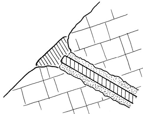
Figure 2. Embedded nail (free condition).
