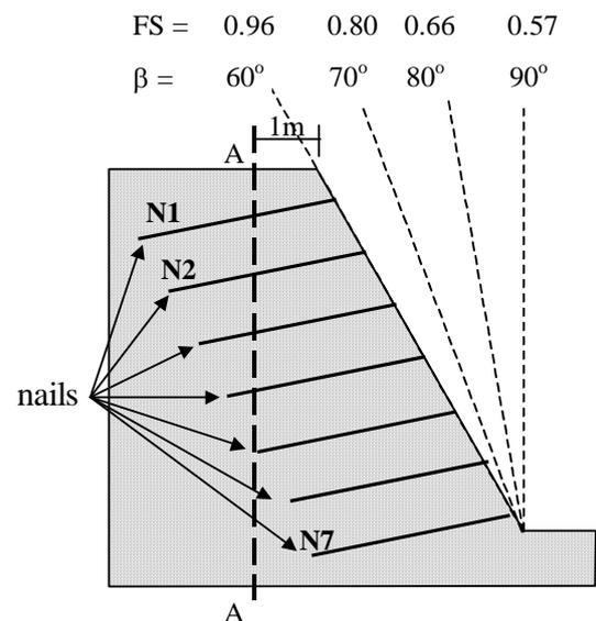
Figure 4. Excavation scheme and safety factors for different slope angles
