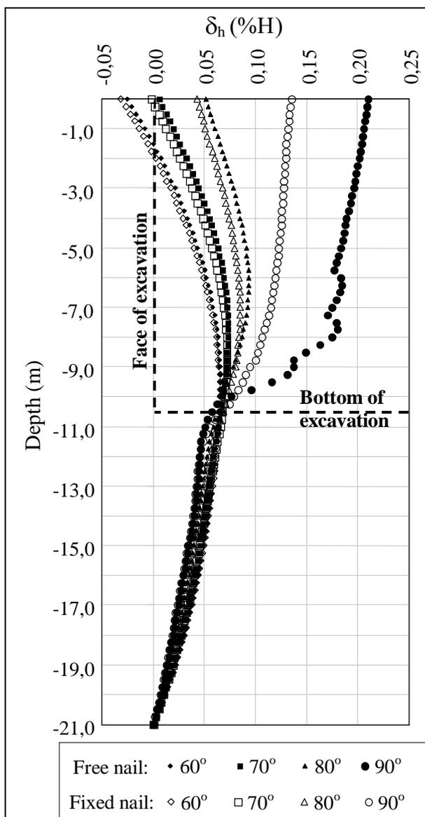
Figure 5. Horizontal displacement profiles
