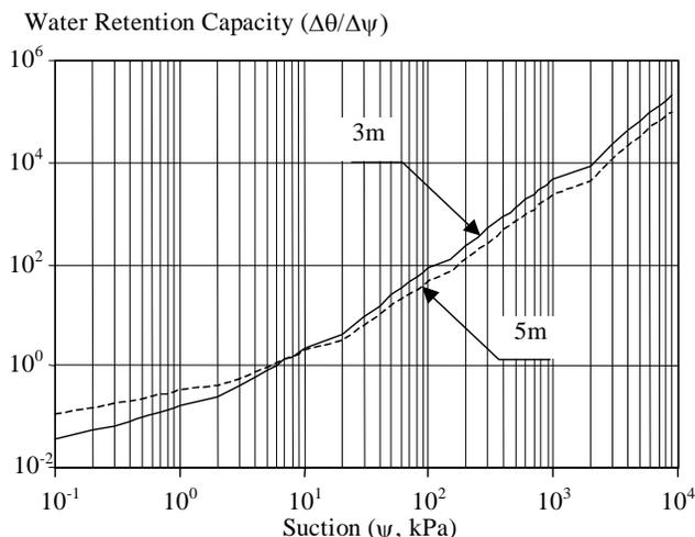
Figure 5. Water retention capacity - São Carlos sedimentary soil at different depths (3m-Test #9 and 5m-Test #10).
