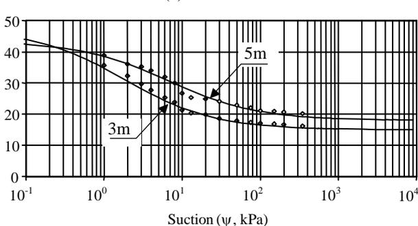
Figure 4. Soil-water characteristic curves - São Carlos sedimentary soil at different depths (3m-Test #9 and 5m-Test #10)
