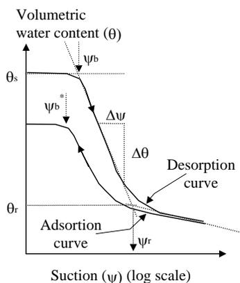
Figure 2. Soil-water characteristic curve parameters.
