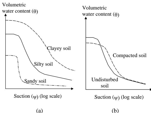
Figure 1. Typical soil-water characteristic curves: (a) Influence of grain size distribution; (b) Influence of soil structure.
