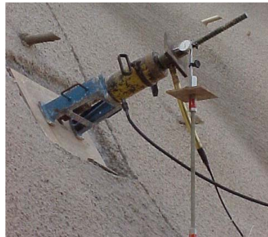
Figure 4 - Pullout test set-up.
